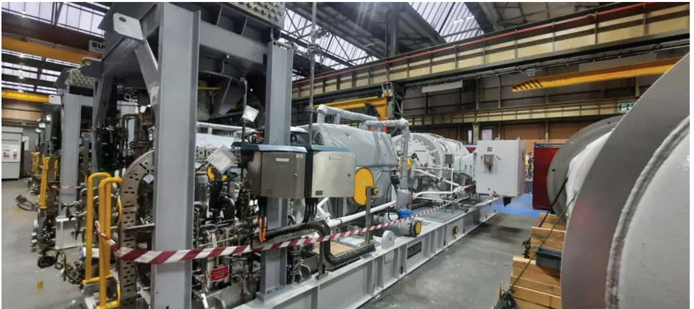
One of the crude oil export pumps for the EACOP being tested at the manufacturing facility
