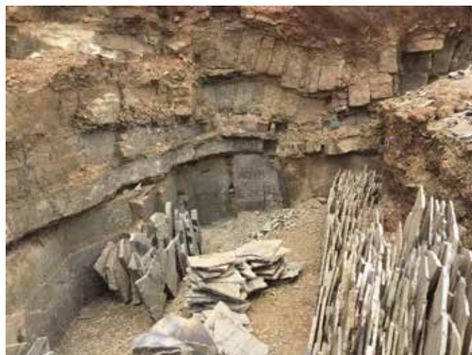
Maji ya Chumvi siltstones are mined for use as dimension or decorative stone
