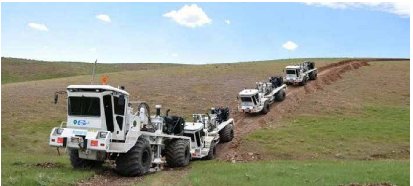
Seismic data acquisition in Eyasi Wembere rift basin.
